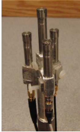
Figure 2.11. Four 6.35 mm microphones mounted in a regular tetrahedral arrangement.
